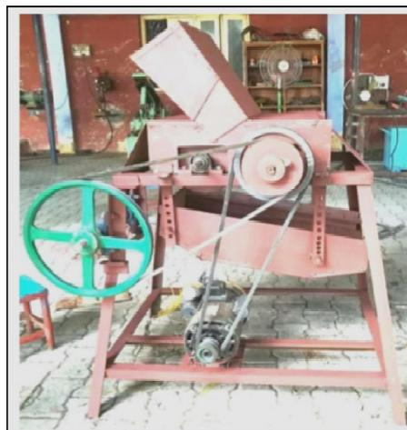
**Fig. 3. Power operated portable sesame thresher**
